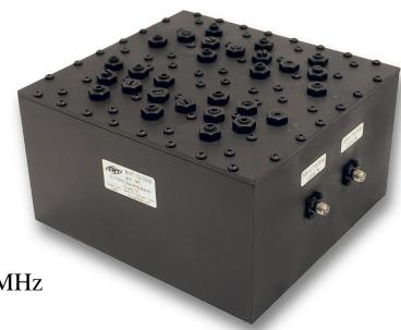
EWT-12-0232 is from a family of filters and duplexers designed for LTE applications. Featuring low IMD products, this model has passband frequencies of 698-716 MHz and 728-746 MHz and exhibits typical passband insertion loss of 1.25 dB with passband return loss of 20 dB. The co-channel isolation is > 60 dB.
